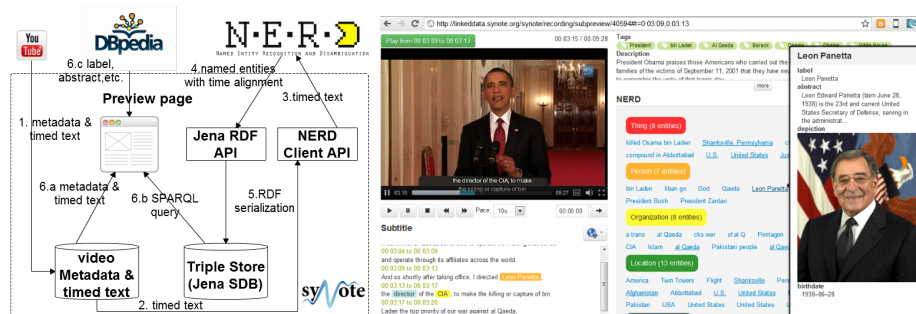
Fig. 1. a) Synote and NERD integration architecture. b) The Synote UI enriched with NERD and DBpedia.
